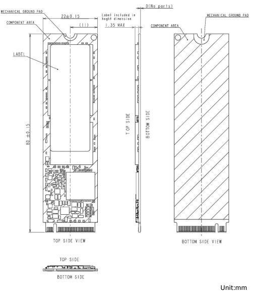
Figure 1: Dimension of KXG5xZNVxxxx (M.2 2280-S2 Module)
